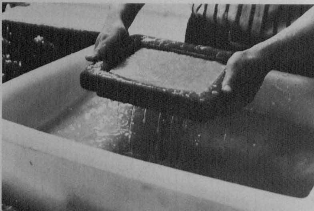
5. Forming the sheet with mold and deckle in the vat; shaking the mold to integrate and mesh the fibers as the water drains through the mold from the pulp.
