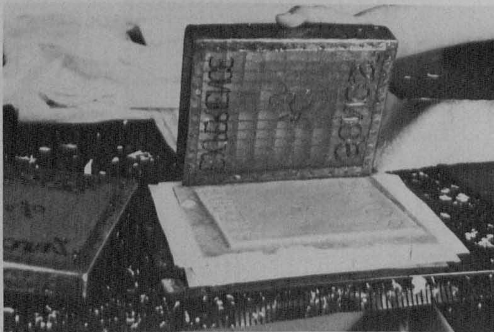
6. Couching the sheet, i.e., transferring the sheet of pulp from mold to felt; the pulp at this stage is very hydrated, and therefore the sheet is very thick. The watermark wires have impressed themselves in the pulp to produce the watermark.
