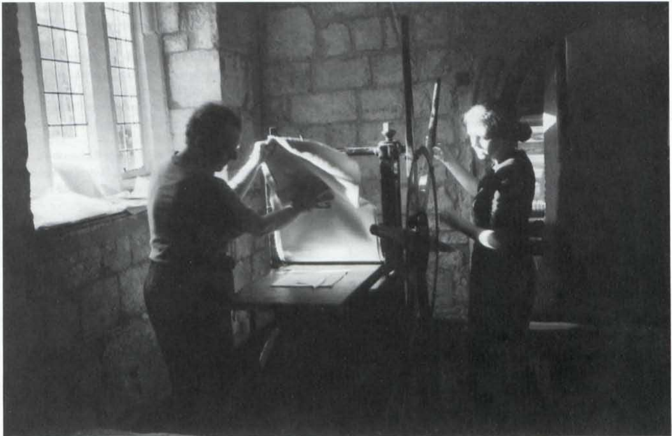
1. Rebecca Minnitt and Michael Phillips printing a relief-etched plate on a star-wheel rolling press, the King's Manor, York, autumn 2000 (photograph by Troy Patenaude).
